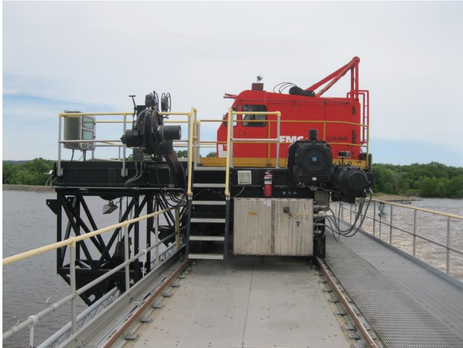
Figure 26–7. Bridge crane installed on an undercarriage
