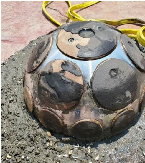
Figure 3–9. Failed pintle ball at Peoria Lock
