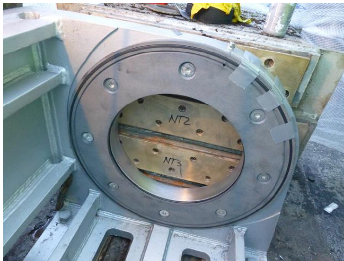
Figure 3-3. Fiber-reinforced plastics trunnion thrust washer installation
