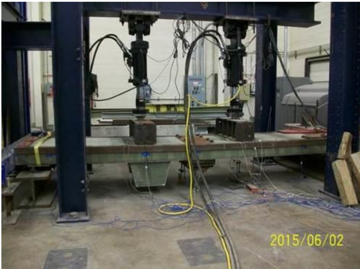
Figure 24–14. Testing prototype composite wicket under bending
