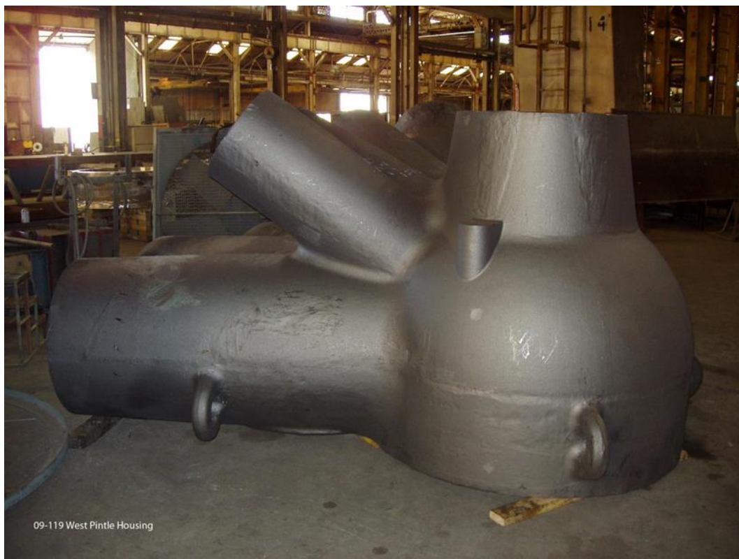
Figure 7–10. West Closure pintle housing
