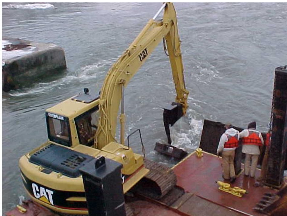
Figure 24–4. Another modified excavator for operating manual wicket gates
