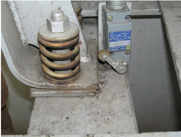
Figure 2–30. Chain guard limit switch in tripped position
