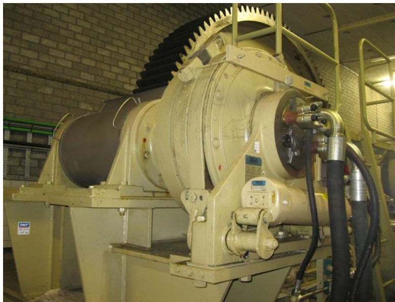
Figure 10–16. Wire rope winch drive at North lock, IJmuiden, Netherlands
