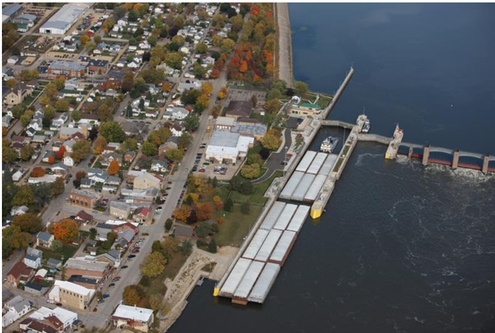
Figure 12–1. USACE – Typical 3-barge-wide and 15-barge tow configuration
