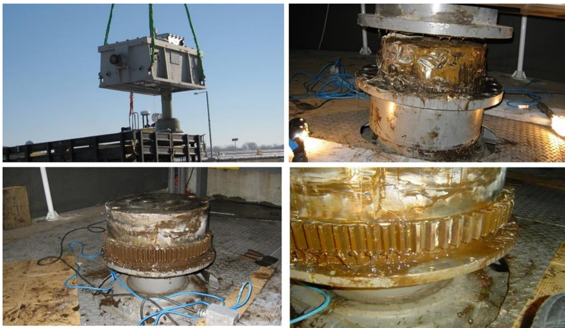
Figure 2–13. Gear-type coupling, Lock 2, Mississippi River
