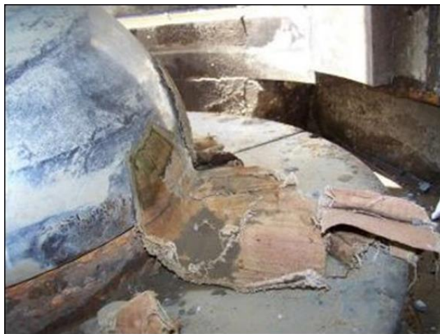
Figure 3–10. Failed pintle at McAlpine Lock
