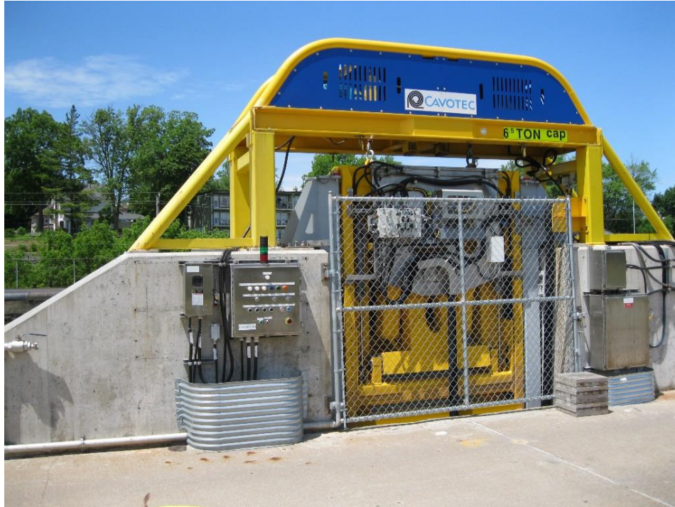
Figure 25-3. Welland Canal Lock 7 hands-free mooring system
