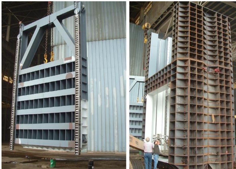
Figure 8–9. Marmet Lock Stoney valve
