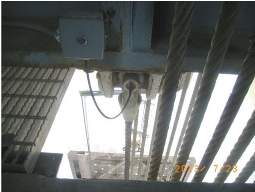
Figure 2–17. Load pin on the anchored end of wire rope
