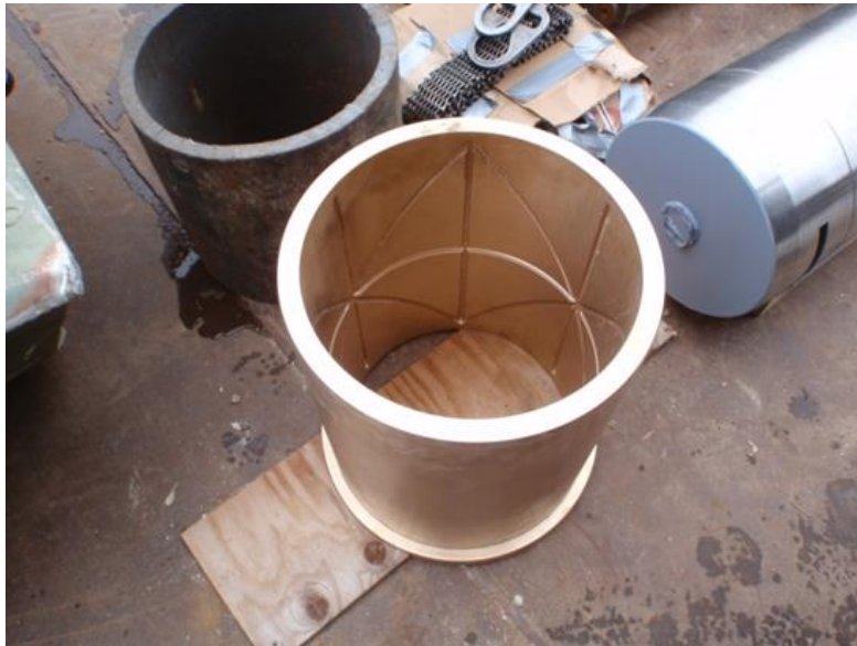
Figure 2–2. Plain bearing for a tainter gate connection
