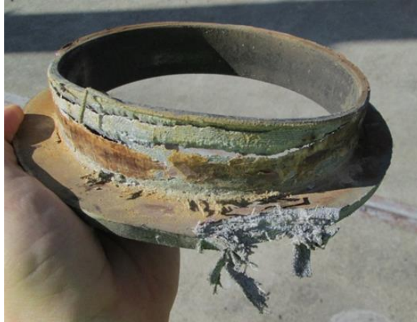
Figure 3-4. Brittle failure of fiber-reinforced plastics self-lubricating gudgeon pin bushing at The Dalles Dam in Portland District
