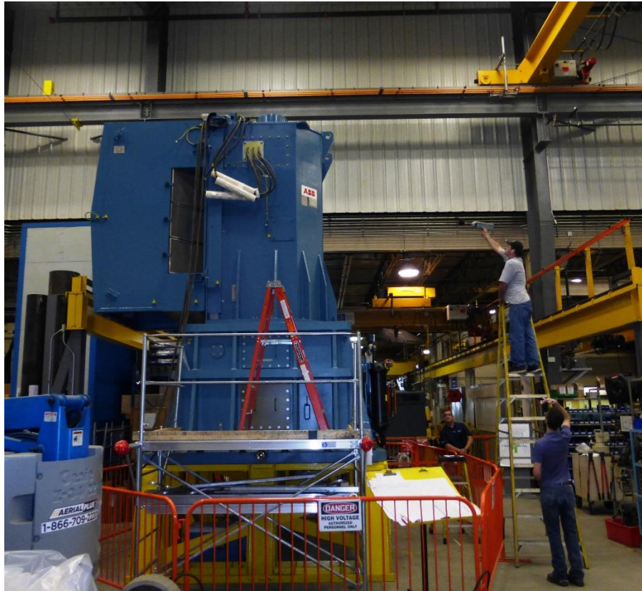
Figure 28–2. Factory testing of pump gearbox
