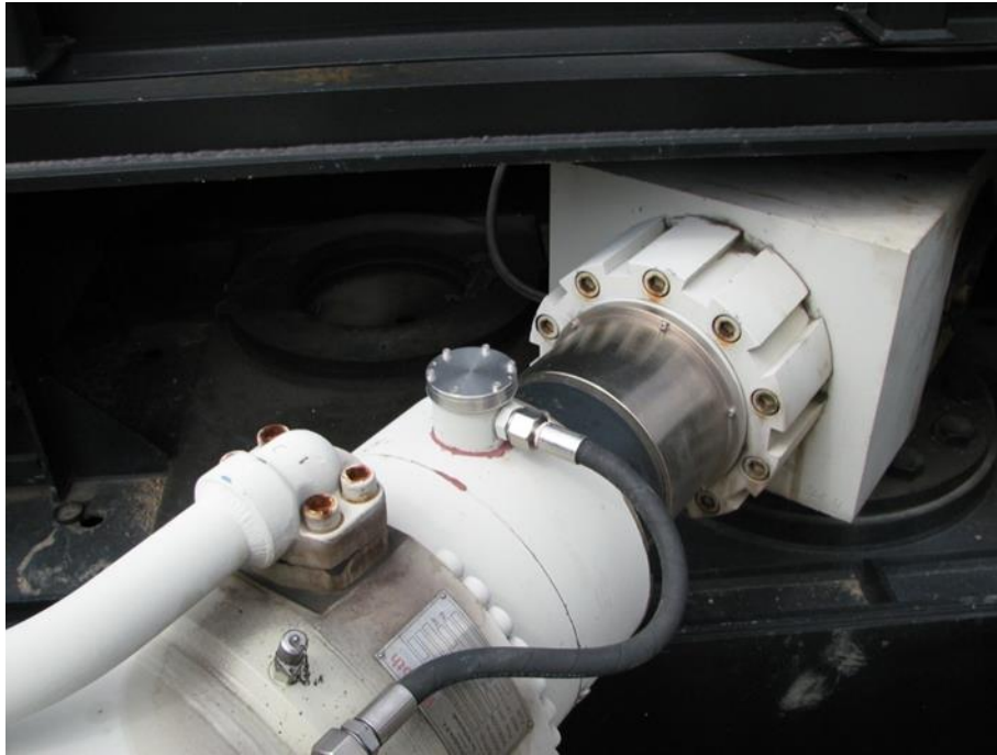
Figure 5–5. Magneto-resistive position sensor on rod end gland
