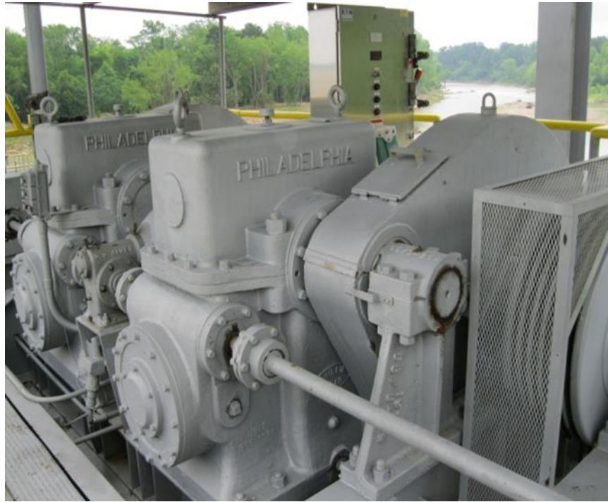
Figure 11–12. Wire rope electric motor hoist
