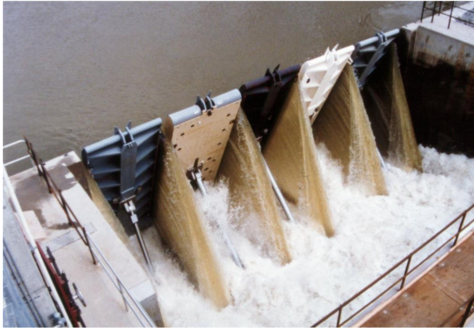
Figure 24-13. Full-scale Olmsted Dam wicket gate prototypes (showing retractable hydraulic cylinder and direct-connect cylinder styles)
