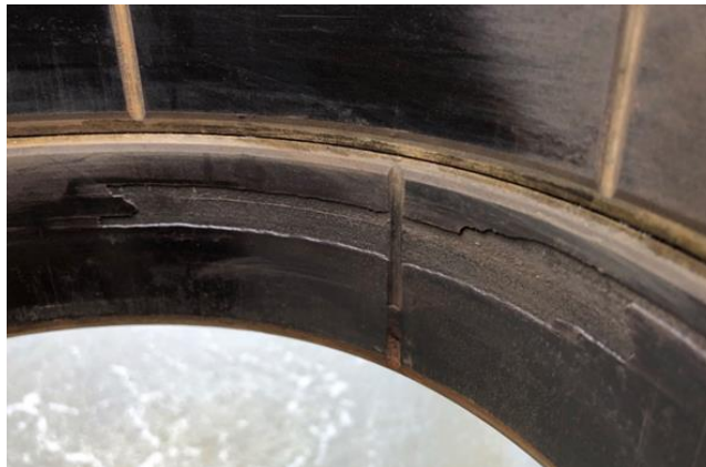
Figure 3-5. Chipped thermal coating on self-lubricating gudgeon pin bushing at Lock and Dam 2 in the St. Paul District
