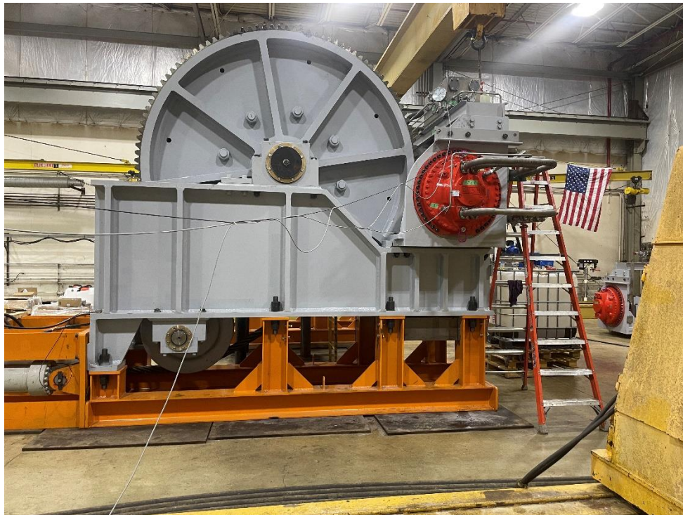
Figure 23–6. New Poe ship arrestor mounted on test rig
