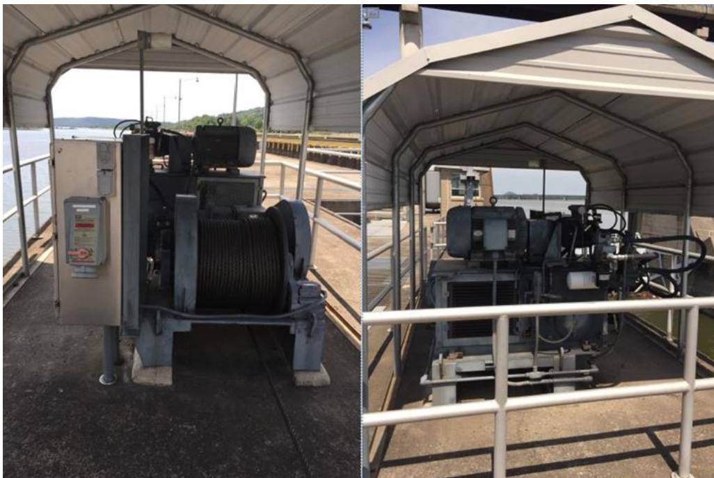
Figure 12-10. Murray Lock – torque-control tow haulage winch with hydraulic power unit
