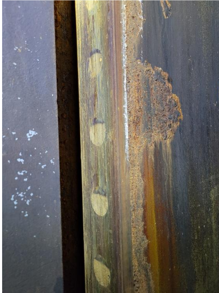
Figure 9–19. Uneven wear on seal screws
