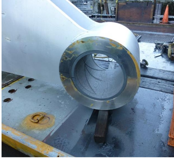
Figure 3-2. Fiber-reinforced plastics trunnion hub installation
