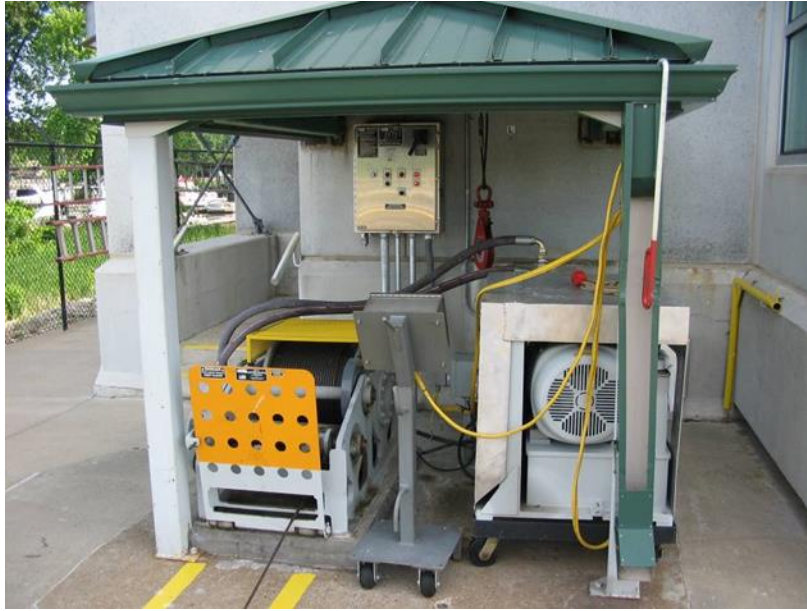
Figure 12–13. Hydraulic-operated tow haulage unit with level-wind system
