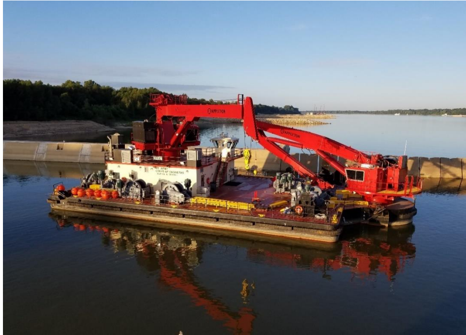
Figure 24–5. Wicket lifter vessel at Olmsted for operating manual wicket gates
