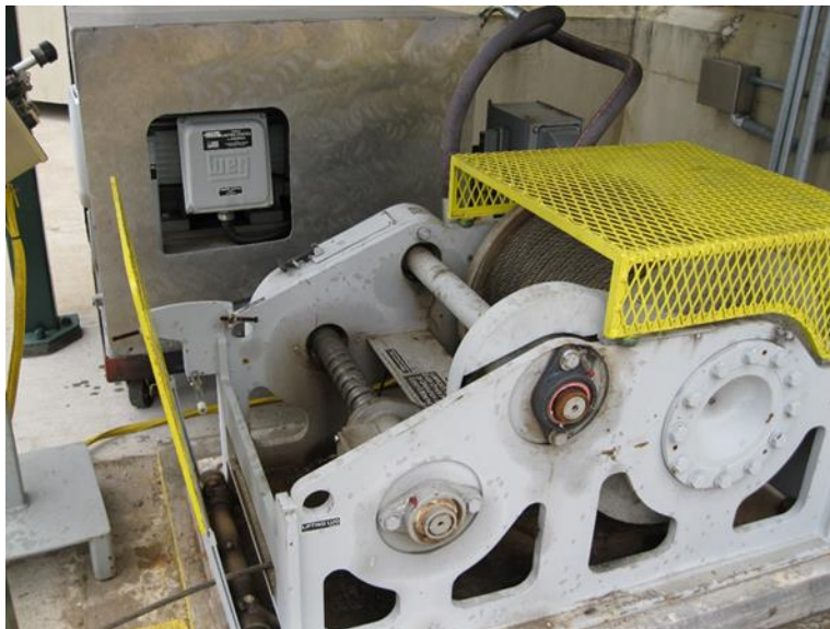
Figure 12–12. Mechanical winch unit with level-wind system
