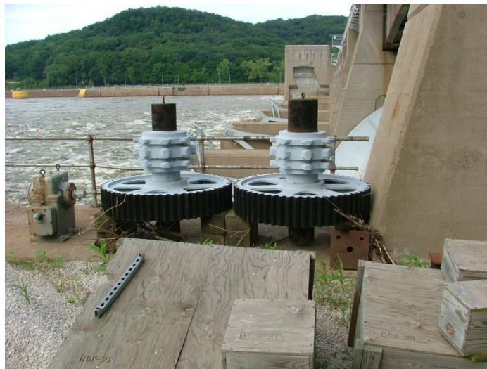
Figure 2–25. Dual chain pocket wheels with spur gear
