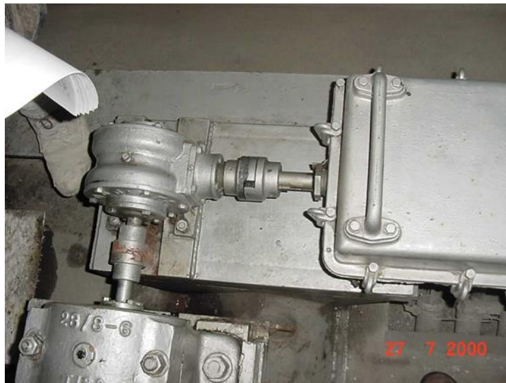
Figure 2-15. Jaw-type coupling detail
