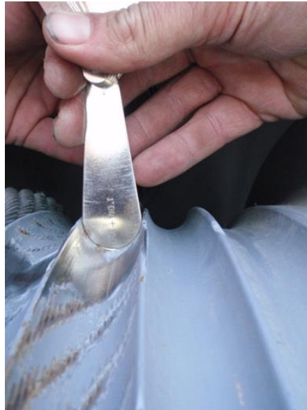
Figure 2-35. Checking wire rope drum groove profile
