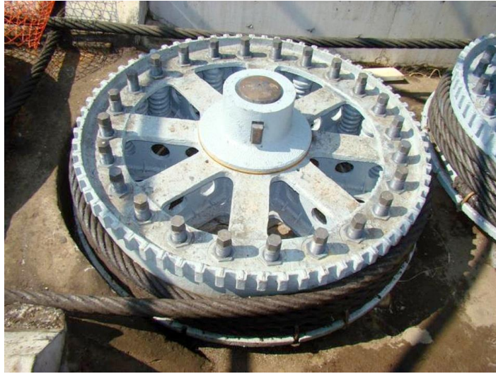
Figure 23–10. Typical brake drum and compression springs, Niagara Region, Lock 6
