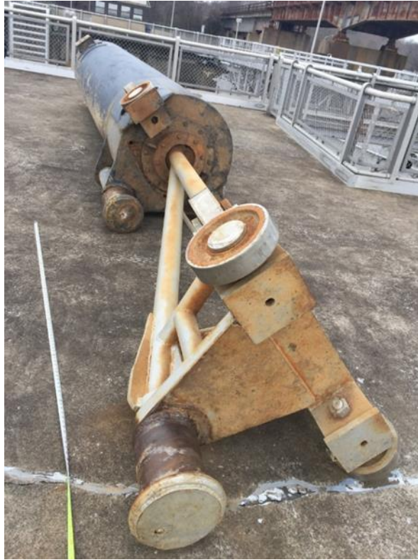
Figure 12–33. Barkley Lock – double-post floating mooring bitt with rollers (old design)
