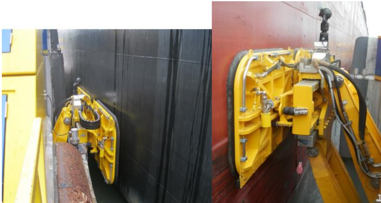
Figure 25–1. Hands-free mooring at St. Lambert Lock, Saint Lawrence Seaway, and Snell Lock
